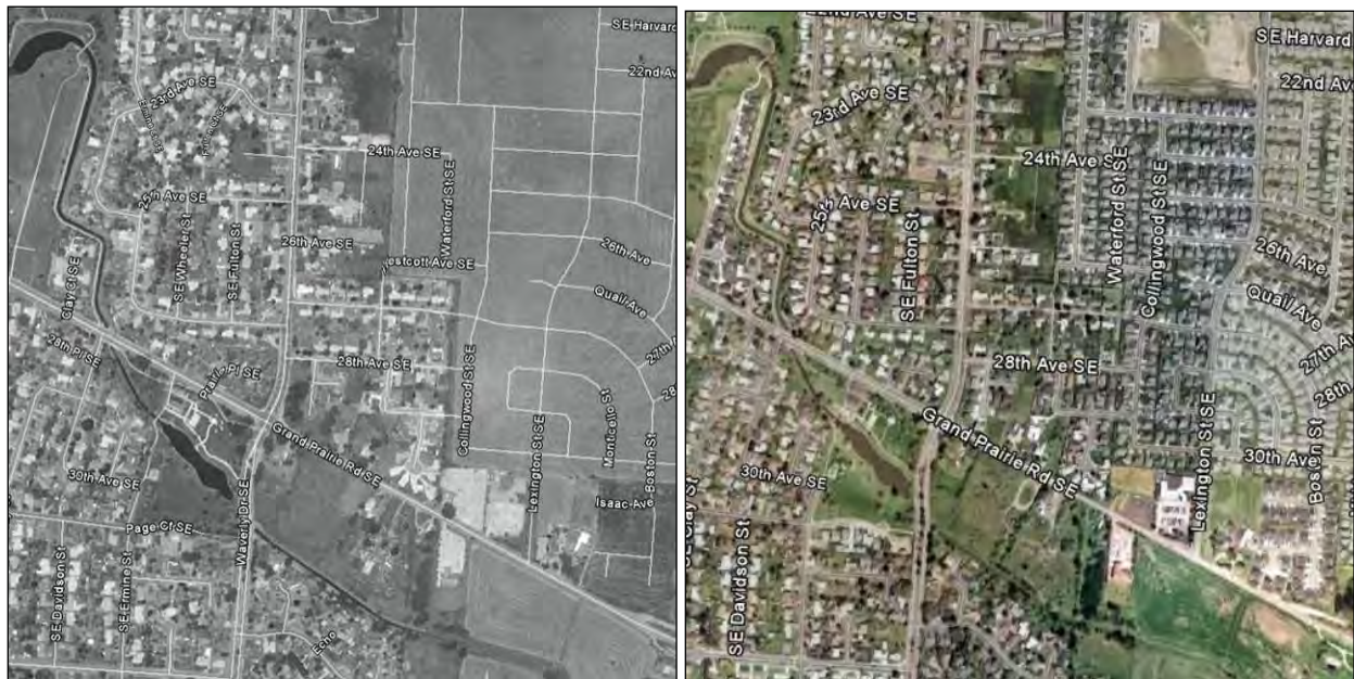
Figure 4-21. A comparison of more recent air photos shows the increasing density of development in the middle Periwinkle Creek watershed. The two air photos from 1994 (left) and 2006 (right) highlight the stream corridor modifications that have occurred on Periwinkle Creek. Infill development that occurred over the 12 years covered by the air photos increased impervious surface area and stormwater discharge.
