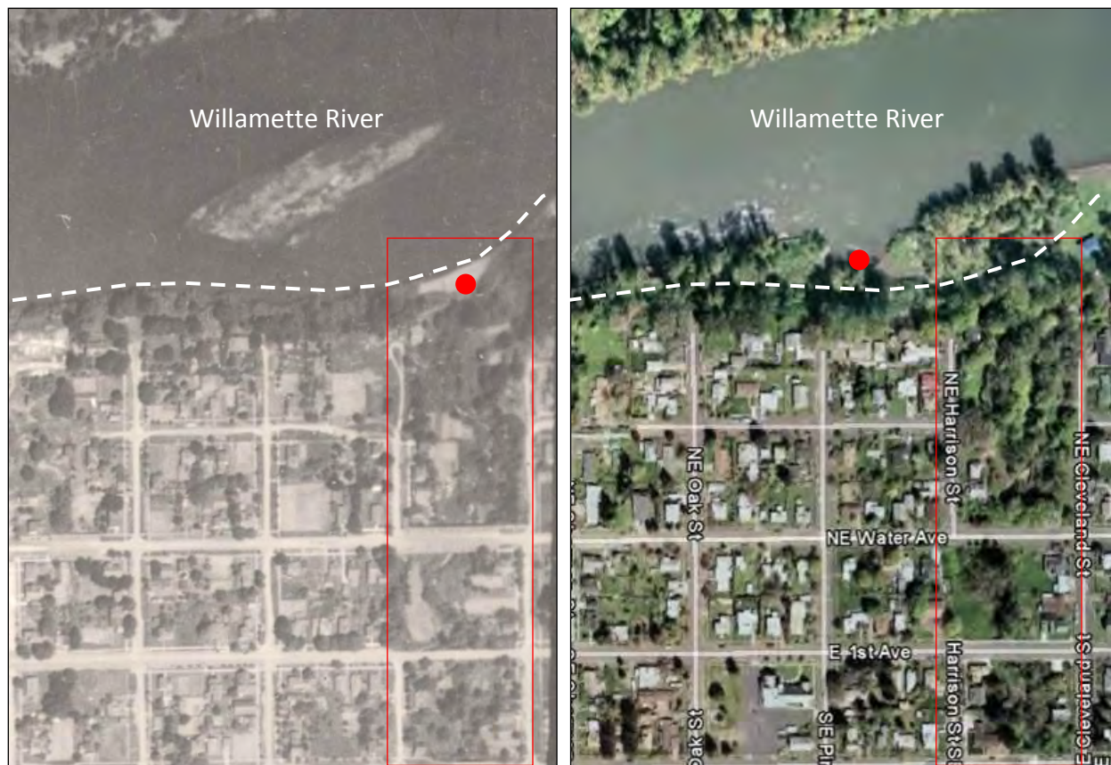
Figure 4-20. A comparison of the 1936 (left) and 2006 (right) air photos of lower Periwinkle Creek. The photos are approximately the same scale and perspective. The red box surrounds the creek in both photos. An island was formerly located mid-channel in the Willamette River across from the Periwinkle Creek confluence. An area that was formerly inundated by the Willamette River, is now floodplain marking the mouth of Periwinkle Creek and the western extent of Bowman Park. The white hatched line shows the 1936 shoreline overlaid on both photos. The red dot represents the Periwinkle Creek confluence.
