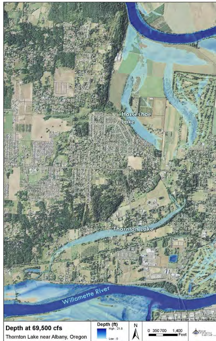
Figure 4-28. The predicted 2-year inundation map for the Willamette River including Thornton Lake and Horseshoe Lake. The Willamette River backwaters into Thornton Lake during the 2-year event, and likely more frequently.
