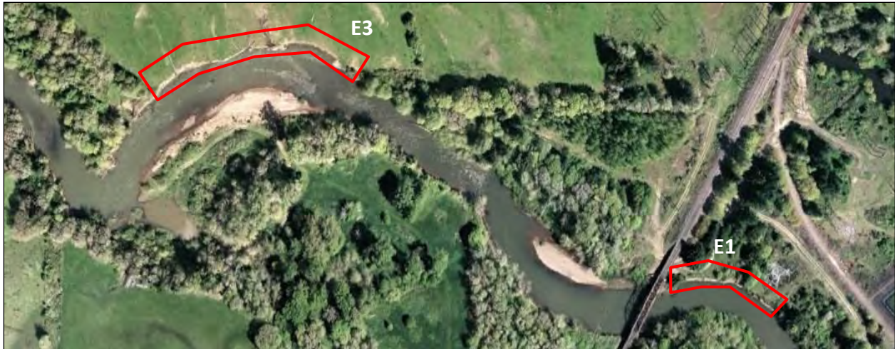
Figure 4-9. The location of E1 and E3 on the Calapooia River. Both sites are located on outside bends. The river is migrating down-valley at E3. Vegetation removal at both sites for power line protection, is likely influencing channel stability.
